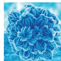
Nanostructure of silicon carbide grown from droplets of gallium on a silicon surface
