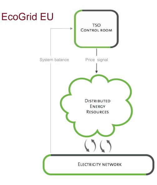
The market concept allows regulation of price signals without direct measurement of the individual DER response
